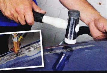
The system is excellent but sometimes other sections get pulled up along with the dent. If this happens, they have to be knocked back down. Sometimes it's appropriate to hit them down while the puller is still applying tension. If there isn't sufficient strength surrounding the dent to be pulled, extra bracing will be required. A slide-hammer attachment can be used to do finer finishing over the damaged area.
